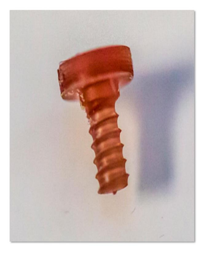
A silk fibroin screw fabricated with golden nanorods can be heated to 160 C when exposed to infrared light emitted by an LED. Credit: Silklab, Department
