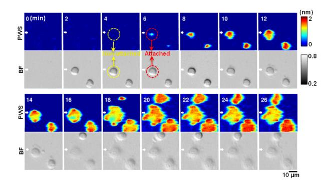
Label-free and dynamic detection of stem cell adhesion uses the photonic crystalenhanced microscope. Credit: Yue Zhuo, University of Illinois
