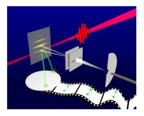
Experimental setup: The helium molecules are produced in a gas jet at an extremely low temperature and separated from the rest of the gas jet in a diffraction grating. The X-ray flash (red) of the FLASH laser (Hamburg) ionises both helium atoms of the molecule so that they fly apart with explosive force. The ions are then mapped on a spatial resolution detector, as symbolized by the film strip. Credit: AG Dörner
