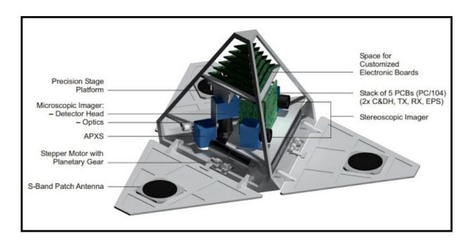
A US-German team of researchers has proposed developing a microscale, low-cost surface lander for the in situ characterization of an asteroid. The tiny spacecraft, called the Pico Autonomous Near-Earth Asteroid In Situ Characterizer (PANIC), could be a breakthrough for the scientific community, offering a simple, cheap solution for asteroid research.
