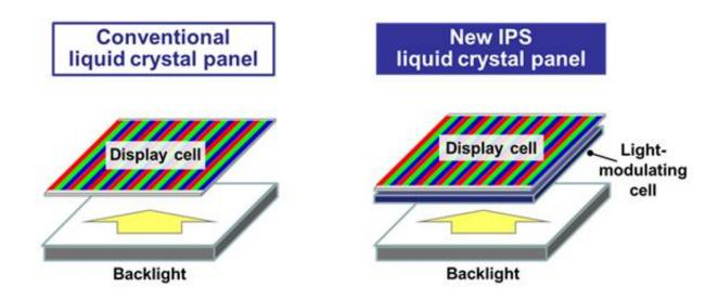
Structural comparison between conventional and new liquid crystal panels. Credit: Panasonic
