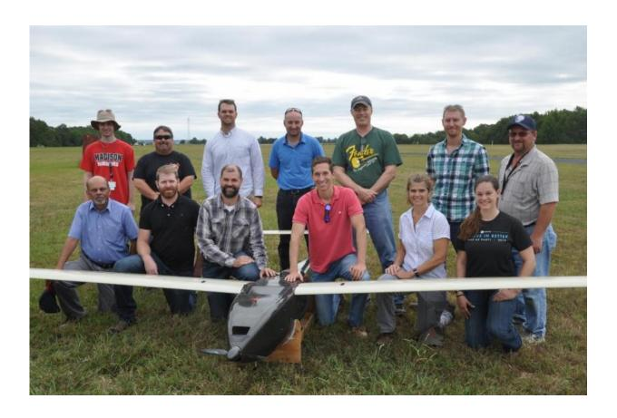
Members of the chemistry and tactical electronic warfare divisions from the U.S. Naval Research Laboratory with the Ion Tiger unmanned air vehicle, which recently flew with a new, custom hydrogen fuel cell designed and built at NRL. The fuel cell system is capable of 5,000 watts and is made of formed and laser-welded metal foil bipolar plates, which saves space and weight. Credit: Naval Research Laboratory
