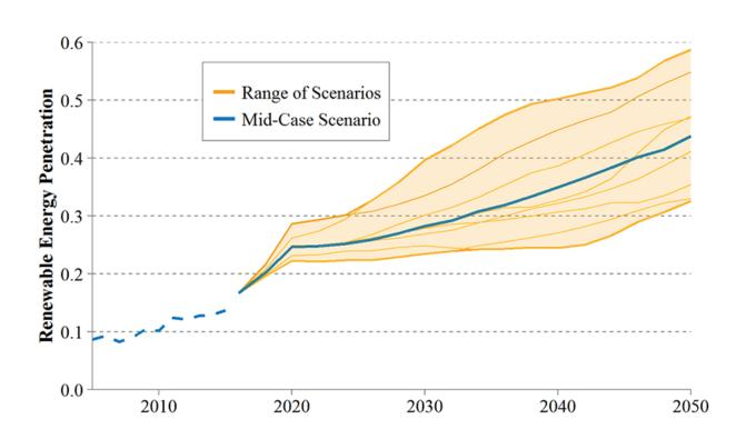
Renewable energy penetration in the U.S. power sector as projected by a subset of the Standard Scenarios, where the dashed line shows historical values. Penetration is defined as the fraction of load met by renewable energy. Credit: NREL.
