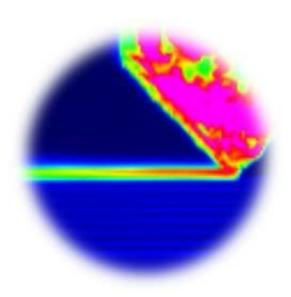
IR thermography measurement of materials extrusion additive manufacturing. Credit: Jon Seppala
