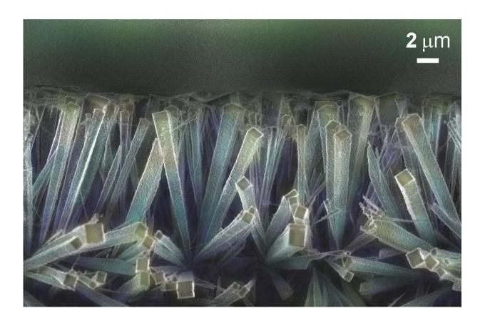
Example of diamond crystallites of different shapes, obtained with the help of the technology, worked out in the Lomonosov Moscow State University. There are electron microscopy images of diamond films' fragments after their oxidation in the air. The material left after the oxidation is represented by needle-like diamond monocrystals of pyramid shape. Credit: Alexander Obraztsov
