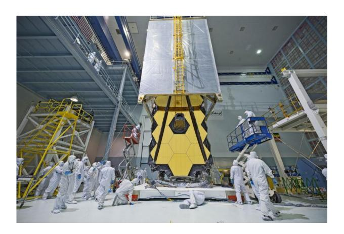
NASA's James Webb Space Telescope placed inside a "clean tent" in Nov. 2016 to protect it from dust and dirt as engineers at NASA's Goddard Space Flight Center in Greenbelt, Maryland transport it out of the relatively dust-free cleanroom and into a shirtsleeve environment to conduct vibration and acoustics tests to confirm it is fit for launch in 2018. Credit: NASA/Chris Gunn
