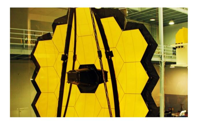
The 18-segment gold coated primary mirror of NASA's James Webb Space Telescope is raised into vertical alignment in the largest clean room at the agency's Goddard Space Flight Center in Greenbelt, Maryland, on Nov. 2, 2016. The secondary mirror mount booms are folded down into stowed for launch configuration. Credit: Ken Kremer/kenkremer.com
