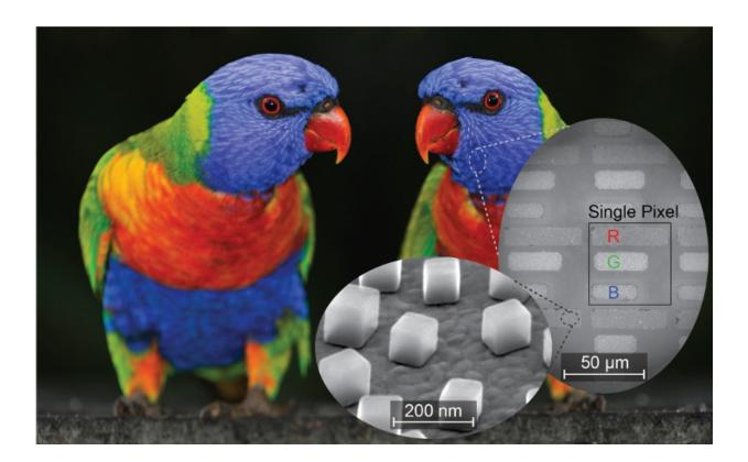
Researchers tested a new technique for printing and imaging in both color and infrared with this image of a parrot. The inlay shows how a simple RGB color scheme was created by building rectangles of varying lengths for each of the colors, as well as individual nanocubes on top of a gold film that create the plasmonic element. Credit: imageBROKER / Alamy Stock Photo
