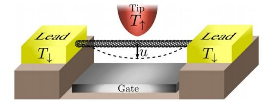
In the proposed system, a carbon nanotube is suspended between two leads, below a tip electrode, and above a gate. The pair of leads and the tip are two separate electron reservoirs with different temperatures. Electrons can tunnel between the nanotube and the reservoirs. Although electron exchange between the two reservoirs is prevented, electron-electron interaction couples the two reservoirs, allowing for a heat flow. Credit: A. Vikström et al. ©2016 American Physical Society
