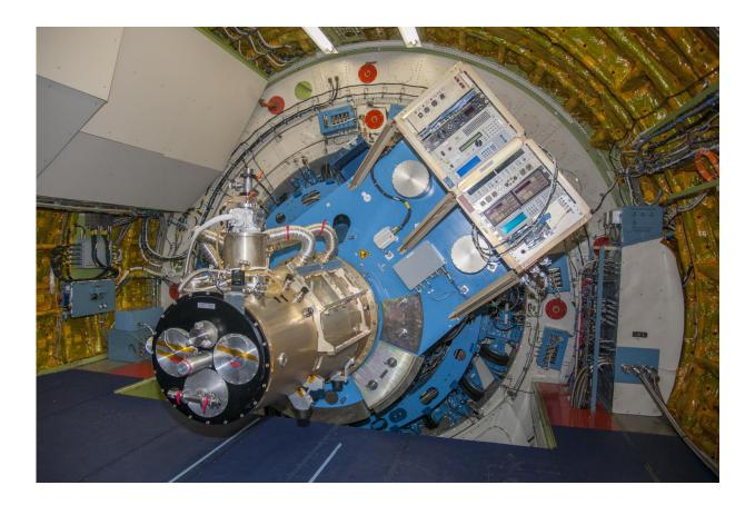
NASA recently completed the commissioning of a new airborne camera on NASA's SOFIA aircraft. This image shows HAWC+ on SOFIA's telescope. Credit: NASA/AFRC
