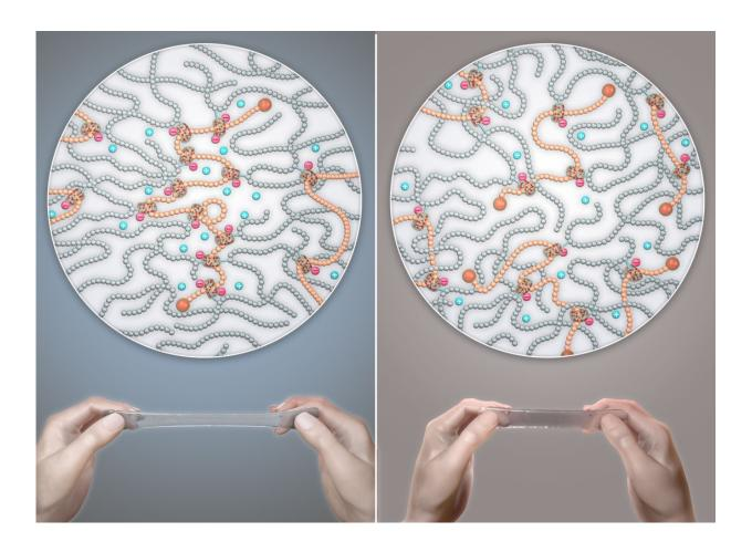
The polymer gels, which were prepared using polyrotaxane (PR) cross-linkers of different molecular weights but the same number of cross-linking points per unit volume of gel, have almost the same Young's modulus. By contrast, the extensibility and rupture strength of the polymer gels are substantially increased with increasing molecular weight of the PR cross-linker. Credit: Yukikazu Takeoka
