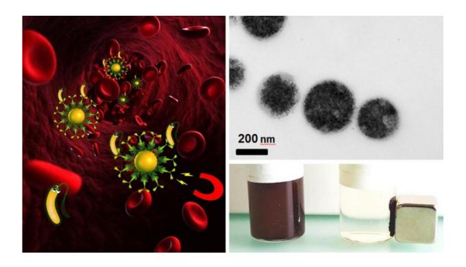
Bacteria can be removed by magnetic blood purification (left). A suspension with magnetic iron particles (top right) can be "cleaned" using a magnet (bottom right). Credit: Laboratory for Materials Science and Technology
