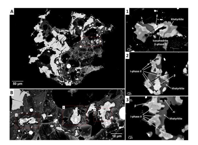
(A) Grain 126A; red dashed box indicates the region to be enlarged in (B). (B) The area where there are the three metal assemblages containing the two different icosahedral phases; red dashed boxes (indicated as 1, 2 and 3) indicate the regions to be enlarged in panels on right. Panels 1, 2 and 3 show the different associations of minerals in the three metal assemblages. Credit: *Scientific Reports* (2016). DOI: 10.1038/srep38117
