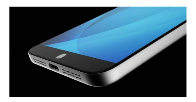
Synaptics today announced an industry-first family of Natural ID biometric authentication solutions that leverage high-performance, highly secure optical-based fingerprint sensors for smartphones and tablets. The new Synaptics FS9100 optical fingerprint sensor family is capable of high-resolution scanning through 1mm of full cover glass and enables clean, button-free industrial designs.
