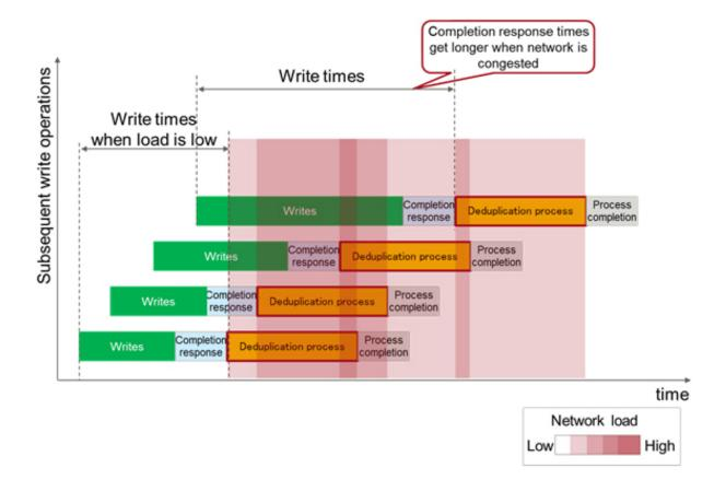
Figure 3: Network load leading to drop in write response speed. Credit: Fujitsu
