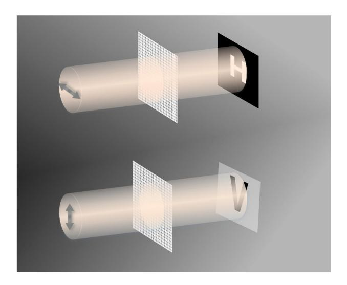
A new technique can be used to hide multiple images in a printed array of rods with varying conductivities. Depending on the polarization of the terahertz radiation, different concealed images appear, such as the H and V illustrated here. Credit: Ajay Nahata, University of Utah
