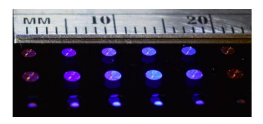
Flat lenses created by combining two layers of metamaterial studded with silicon nanoposts. Credit: Caltech
