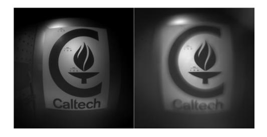
Two layers of nanoposts yields a wider field of clarity (left), compared to a single layer (right). Credit: Caltech
