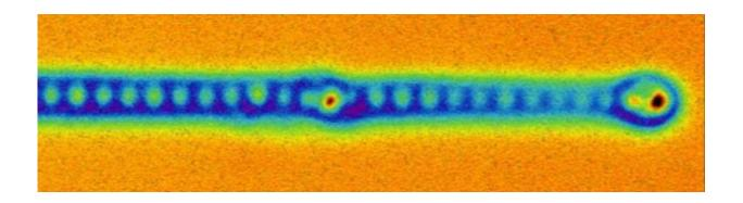
Atomic force microscopy image of the end of a mono-atomic iron wire. The individual iron atoms are clear to see, as well as the "eye" of the Majorana fermions on the end. Credit: University of Basel, Department of Physics
