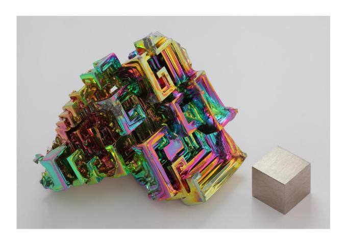
Artificially grown bismuth crystal illustrating the stairstep crystal structure, with a 1 cm3 cube of bismuth metal. Credit: Wikipedia
