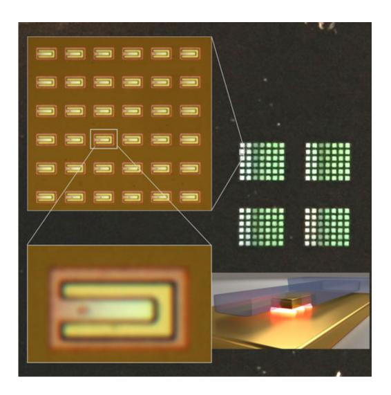
These optical micrographs provide a top-down view of several plasmonic gap resonators and zoom in on a single device. Bottom right shows schematic of a single device. Credit: NIST Center for Nanoscale Science and Technology
