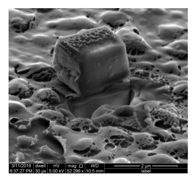
An isolated cement cube created by the lab of Rice materials scientist Rouzbeh Shahsavari. Microscopic cubes and other shapes may serve as 'seeds' in programmable cement for stronger, less porous and more environmentally friendly concrete. Credit: Multiscale Materials Laboratory/Rice University
