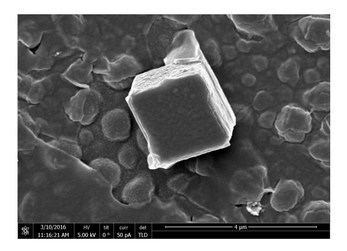
Rice University scientists created microscopic cubes and other shapes of cement and crushed them to test their mechanical properties. The shapes may serve as 'seeds' for the bottom-up manufacture of stronger, more durable concrete. Credit: Multiscale Materials Laboratory/Rice University
