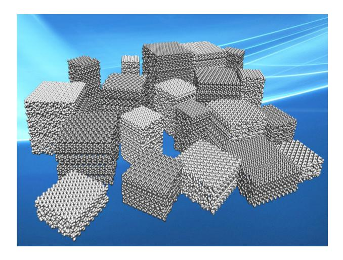
Rice University materials scientists have mapped the morphogenesis of cement hydrates used in concrete. It could lead to a way to 'program' cement particles for the manufacture of stronger, more durable and more environmentally friendly concrete. Credit: Multiscale Materials Laboratory/Rice University
