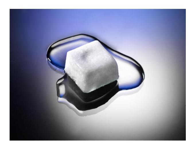
The PCM cube maintains a temperature of 21 degrees Celsius until it is completley melted. Credit: Fraunhofer ICT
