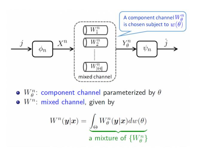
The coding system over mixed channels with general mixture. Credit: University of Electro-Communications
