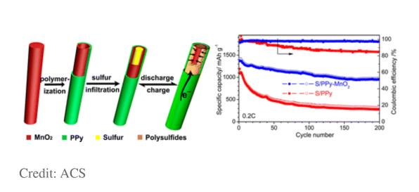
(Phys.org)—A team of researchers at the University of Texas has found that using coaxial nanotubes can improve the performance of lithium-sulfur batteries (Li-S). In their paper published in the journal *Nano Letters*, the team describes how they used Polypyrrole-MnO<sub>2</sub> coaxial nanotubes to overcome obstacles to using Li-S batteries in commercial products.
