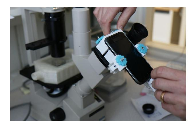
Setting up. The standard inverted microscope is upgraded to a high quality live imaging station. Credit: Linda Koffmar
