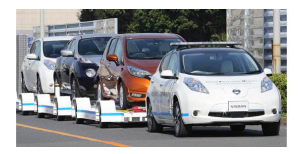
Nissan Motor Co.'S "Leaf", with no one inside, pulls a trailer with three other Leafs on it, during a demonstration of the automaker's Intelligent Vehicle Towing system at Nissan Oppama plant in Yokohama, near Tokyo Monday, Dec. 5, 2016. Nissan Motor Co. is testing out self-driving cars at one of its plants in Japan to tow vehicles on a trailer to the wharf for loading without anyone behind the steering wheel. (AP Photo/Koji Sasahara)
