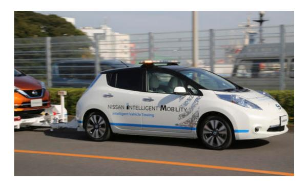
Nissan Motor Co.'s "Leaf" runs with no one inside during a demonstration of the automaker's Intelligent Vehicle Towing system at Nissan Oppama plant in Yokohama, near Tokyo Monday, Dec. 5, 2016. Nissan Motor Co. is testing out self-driving cars at one of its plants in Japan to tow vehicles on a trailer to the wharf for loading without anyone behind the steering wheel.(AP Photo/Koji Sasahara)
