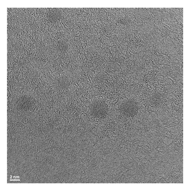
Nitrogen-doped graphene quantum dots stand out from a substrate in a transmission electron microscope image. The dots are effective electrocatalysts that can reduce carbon dioxide, a greenhouse gas, to valuable hydrocarbons like ethylene and ethanol. Credit: Ajayan Group/Rice University
