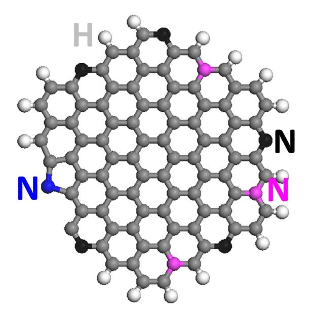
An illustration of a nitrogen-doped graphene quantum dot like those being tested at Rice University for use as catalysts to reduce carbon dioxide, a greenhouse gas, into valuable hydrocarbons. Credit: Ajayan Group/Rice University
