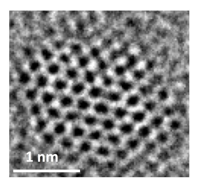
A single nitrogen-doped graphene quantum dot with zig-zag edges. Credit:
