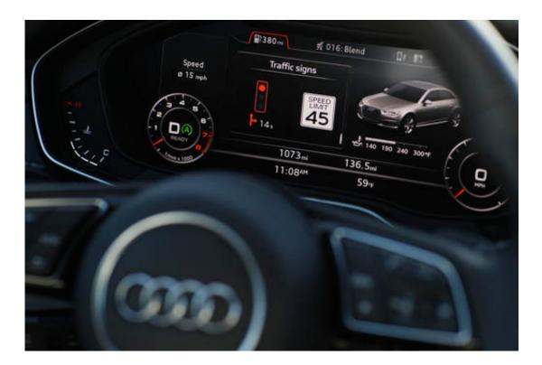
The dashboard of an Audi A4 is seen during a demonstration of Audi's vehicle-to-infrastructure technology Tuesday, Dec. 6, 2016, in Las Vegas. The technology allows vehicles to "read" red lights ahead and tell the driver how long it'll be before the signal turns green. For the driver, the system puts a traffic signal icon on the dashboard telling how many seconds the light will remain red. (AP Photo/John Locher)
