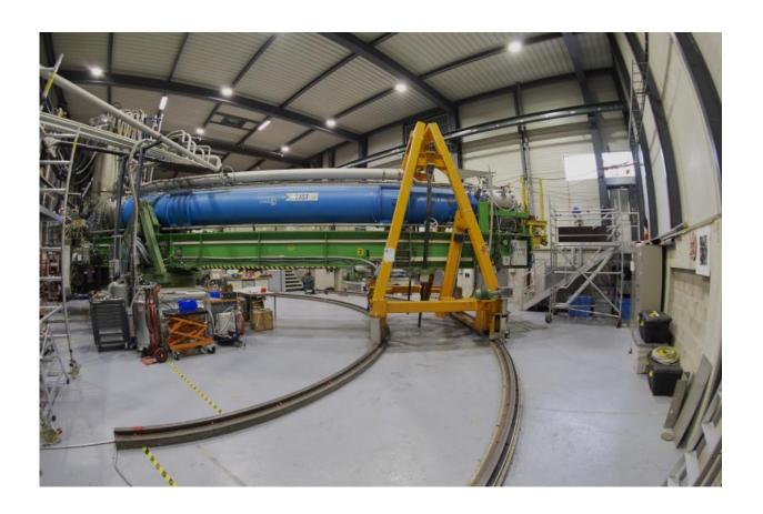
The CAST telescope is made of a prototype dipole magnet from the Large Hadron Collider. It moves along the tracks on the ground to follow the Sun's movement across the sky. Credit: Maximilien Brice/ CERN
