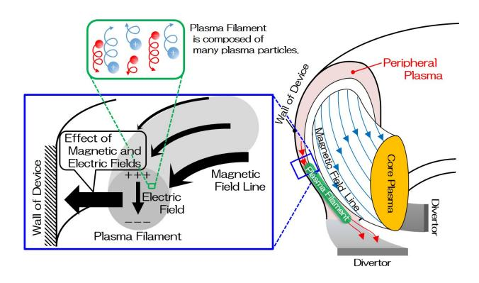
The plasma blob takes a thin and long form and follows the magnetic field lines. This blob is composed of numerous plasma particles (ions and electrons). However, due to the magnetic field lines and the influence of the electrical field inside the plasma, the blob flies in the direction of the confinement vessel wall. Credit: Dr. Hiroki Hasegawa
