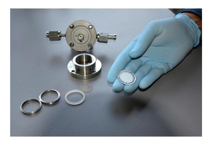
Michael Metzger, researcher at the Technical University of Munich (TUM), shows the core of his new battery test cell: A glass ceramic membrane, coated with aluminum and plastic, allows only lithium ions to pass through. It is impermeable to all other components of the electrolyte fluid, thus allowing to investigate anionic and cationic reactions in lithium-ion batteries separately. Credit: Monika Weiner / TUM
