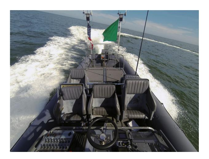
An unmanned rigid-hull inflatable boat operates autonomously during an Office of Naval Research (ONR)-sponsored demonstration of swarmboat technology held at Joint Expeditionary Base Little Creek-Fort Story. During the demonstration four boats, using an ONR-sponsored system called CARACaS (Control Architecture for Robotic Agent Command Sensing), operated autonomously during various scenarios designed to identify, trail or track a target
