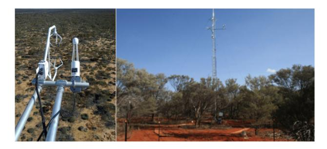
Flux towers for measuring carbon and water fluxes between ecosystem and the atmosphere: (left) Calperum near Adelaide; (right) Alice Springs Mulga woodland in central Australia. Both sites are part of Australia's Terrestrial Ecosystem Research Network, or TERN. Credit: www.ozflux.org.au
