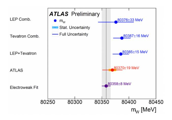
The ATLAS measurement of the W boson mass (in red) is compared to the Standard Model prediction (in purple), and to the combined values measured at the LEP and Tevatron collider (in blue). Credit: ATLAS Collaboration/CERN
