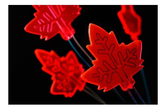
Even with the naked eye the amount of light captured by the 'mini-factories' is visible, lit up bright red. The 'veins' through the leaves are the thin channels through which liquid can be pumped. The start products enter the one channel, light causes the reactions and the end product comes out via the other channels. Credit: TU Eindhoven / Bart van Overbeeke
