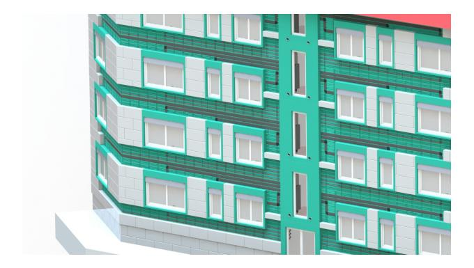
Facade elements that do not only contain thermal insulation, but also heating and ventilation components are in the focus of LowEx-Bestand. Credit: Fraunhofer ISE
