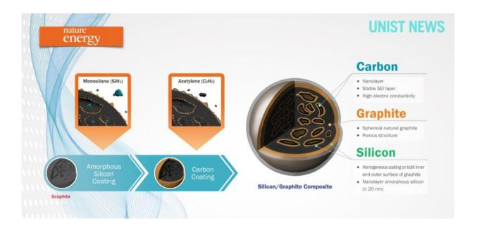
Cross-sectional schematic view showing the detailed structural characteristics of a SGC hybrid particle. Credit: UNIST
