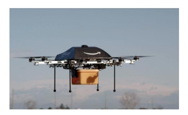
An Amazon picture of a flying "octocopter" mini-drone that would be used to fly small packages to consumers
