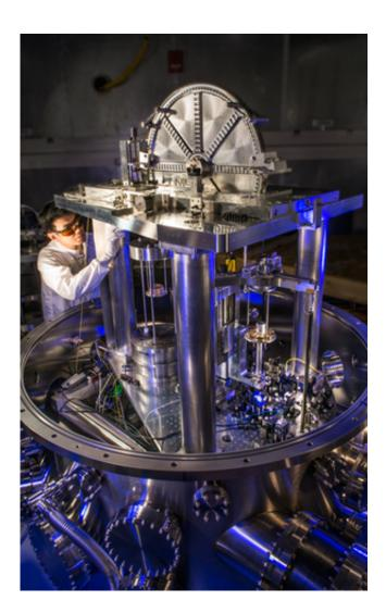
Through its measurements of Planck's constant, a quantity at the heart of quantum physics, the NIST-4 watt balance is contributing to an effort to define all base measurement units in terms of fundamental constants of nature. Credit:
