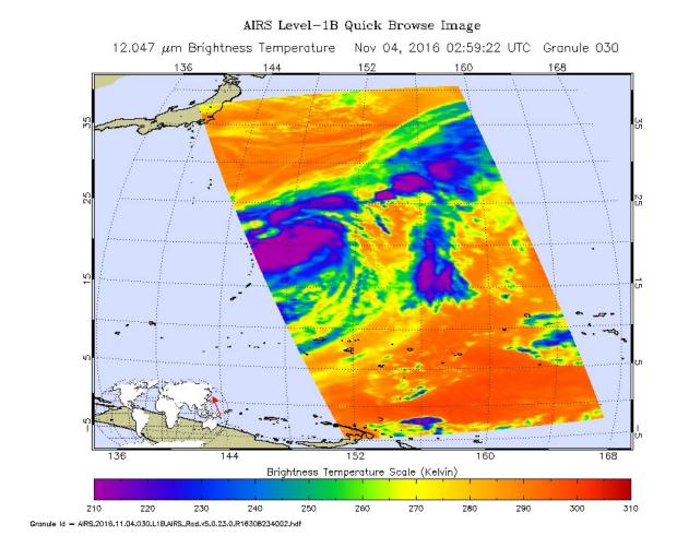
On November 4, 2016, NASA's Atmospheric Infrared Sounder (AIRS) instrument on NASA's Aqua satellite produced this false-color infrared image of Meari as it headed northeast. The image shows the temperature of Meari's cloud tops or the surface of Earth in cloud-free regions, with the most intense thunderstorms shown in purples and blues. Credit: NASA/JPL-Caltech
