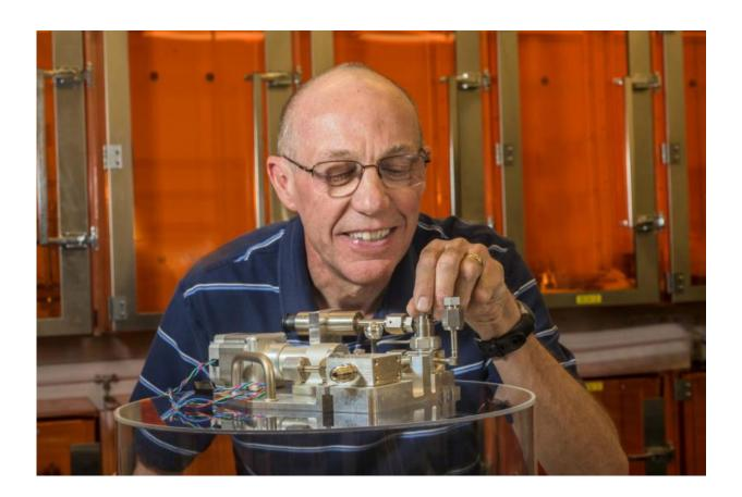
Sandia National Laboratories principal investigator Dean Rovang checks out the Z Machine's tritium gas transfer system, which was built at the labs' Livermore, California, site and filled with trace tritium (0.1 percent) at Sandia in Albuquerque. Credit: Randy Montoya
