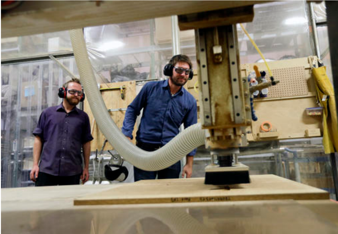
In this Tuesday, Sept. 27, 2016 photo, Ecovative Design co-founder Eben Bayer, right, and prototype engineer Kenneth Lush watch as a pattern is cut from "myco-board" in Green Island, N.Y. (AP Photo/Mike Groll)
