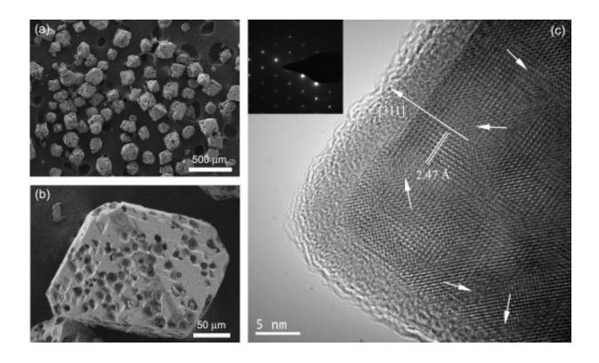
Electron micrographs of tiny superparamagnetic crystals of magnetite at different resolutions. The lowest resolution image (a) shows the octahedral crystals. At higher resolution, the 'craters' on the crystal surfaces are clearly visible. The highest resolution image (c) shows some of the defects in the crystal lattice, highlighted with the white arrows. Credit: Elsevier B.V
