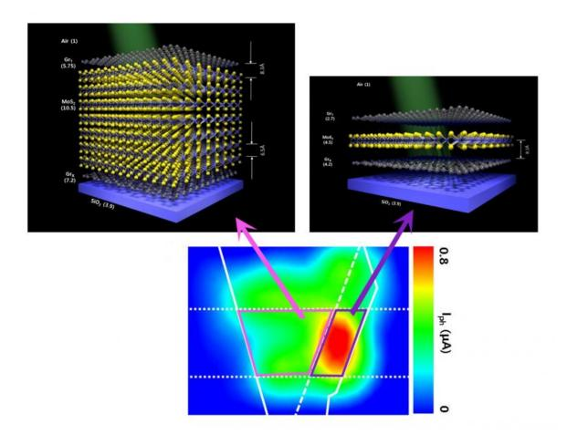
(top) Devices with one-layer and seven-layer MoS2 were built on top of a silicon base and compared. Dielectric constants responsible for the difference in electrostatic potentials are shown in parenthesis. (bottom) The device with one-layer MoS2 (inside the violet box) showed better performance in converting light to electric current than the seven-layer device (inside the pink box). Credit: Institute for Basic Science
