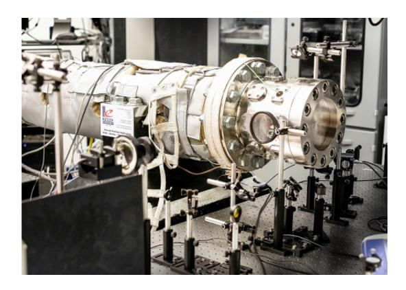
End view of the shock tube used to model the auto-ignition properties of light naphtha. Credit: KAUST
