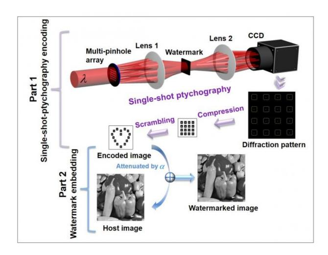
A new optical watermarking system uses single-shot ptychography encoding to create the watermark (Part 1) that is then embedded into a host image (Part 2). Credit: Yishi Shi, University of Chinese Academy of Sciences
