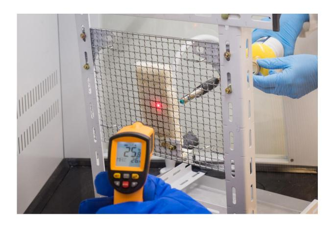
NTU thin foam is subjected to 1,100 degrees Celsius flame from a blowtorch. Its rear remains cool at 26 degrees, demonstrating its effectiveness as a heat insulator and its non-flammable properties. Credit: NTU Singapore
